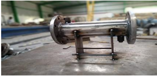
Fig.15. Shell welded with saddle and flanges
